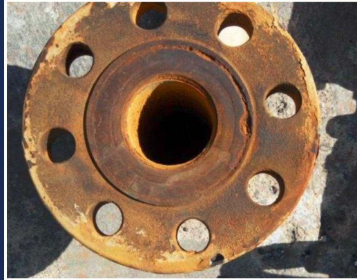
FIGURE 1. A TYPICAL 2" MONEL PLUG VALVE BEFORE CLEANING
