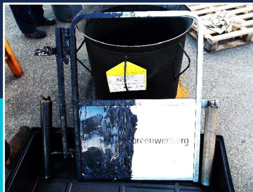
FIG. 6 A GATE FROM THE PROCESS UNIT, BADLY FOULED WITH AN OILY PRODUCT, AFTER 10 MINUTES, HALF SUBMERGED IN THE ULTRASONIC BATH
